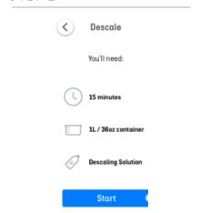
Duration will be 15 mins. Retrieve a 1L container and 1 packet of Nespresso descaling solution.
