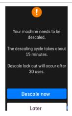
The display will alert the user when it's time to descale. A countdown of 30 uses will begin if bypassed. Select DESCALE NOW.
