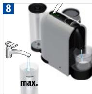
Empty and rinse the water tank, capsule container, drip tray and cup support thoroughly. Fill water tank with potable water. When ready, touch any control to rinse the machine. Machine will stop when done.
