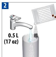
Fill the water tank with 1 unit of Nespresso descaling liquid and add 0.5 L / 17 oz of water.
