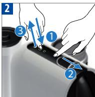
Touch and hold the control while closing the slider. Release control when desired volume is reached. The other 2 controls flash for confirmation.
