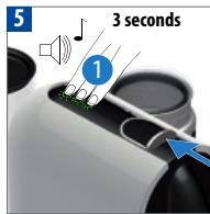
To enter descaling mode, close the slider and press all 3 buttons simultaneously for at least 3 seconds. A short beep will sound to confirm. Open the slider.
