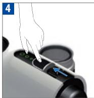
Turn the machine ON by opening the slider and pushing it towards the back of the machine. Light will blink on one of the coffee touch controls: heating up for approximately 25 seconds. Steady light: ready. The machine can be turned into OFF mode at any time when slider is closed by pushing and holding any touch control for more than 3 seconds, confirmed by the other 2 controls flashing.
