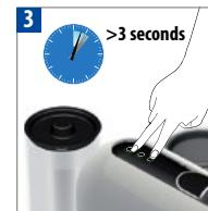
To change automatic OFF mode from 9 to 30 minutes, when slider is closed press and hold both the Lungo and Ristretto controls for more than 3 seconds. Espresso control flashes once for confirmation. To revert back to 9 minutes, repeat the same procedure. Espresso control flashes 3 times for confirmation.
