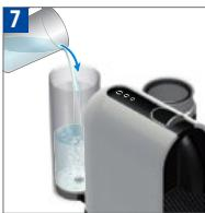
Refill the water tank with the used descaling solution collected in the container and touch any control to repeat the procedure.
