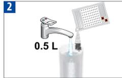
2 Fill the water tank with 1 unit of *Nespresso* descaling liquid and add 0.5 L of water.
