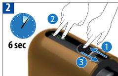
Open slider. Press and hold the Ristretto & Lungo controls together for at least 6 sec. The other control flashes for confirmation. Then close the slider to start procedure.
