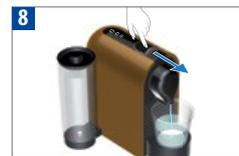
Close the slider to start descaling. Machine stops when water tank is empty.
