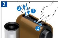
Touch and hold the control while closing the slider. Release control when desired volume is reached. The other 2 controls flash for confirmation. Water volume level is now stored in the control used during programming.
