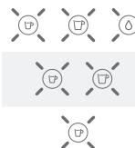
Espresso, Lungo, Hot water blinking: Hard
