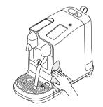
Ory all parts with a soft clean cloth and reassemble machine. Wipe coffee outlet and machine regularly with a clean damp cloth.
