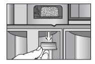
■ Pull the rubber connector downwards.
