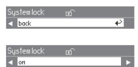
■ Turn the control dial to "on", and then press the control dial to activate the lock.
