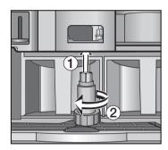
■ Place the special tool (supplied) for removing the capsule hopper on to the brew unit from below and turn the capsule hopper anti-clockwise to remove it.
