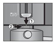
■ Press on the steam valve ① to connect the valve to the milk frother ②.
