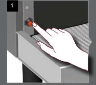
After two hours of non-use, the machine switches to the maximum energy save mode. Press the energy save button to restart.
