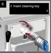
When key inserted cleaning starts automatically.
