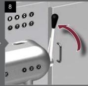
By pulling up the lever, the used capsule list ejected.
