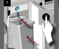
Container must be empty. Afterwards press any button. 8 < Remove cleaning key insert cleaning tablets >
