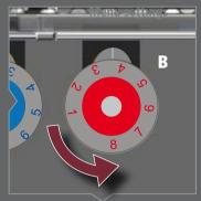
Turn right setting control (B) until air bubbles are visible. Then turn setting control back slightly.
