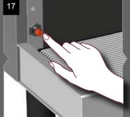
After cleaning process the machine switches to the energy save mode. To restart the machine, press the energy save button.
