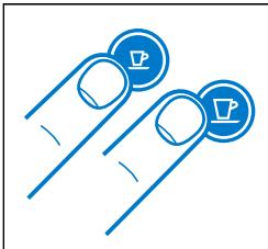
1. To enter the emptying mode, press both the Espresso and Lungo buttons to turn the machine off.
