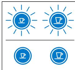
3. LEDs will then continue to blink normally, as heating up, until ready.
