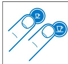
To turn the machine off before automatic Power Off mode, press both the Espresso and Lungo buttons simultaneously.
