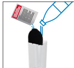
3. Fill the water tank with 0.5 L of potable water and add 1 Nespresso descaling liquid sachet.
