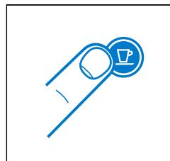
4. To exit the energy saving mode press the Lungo button for 3 seconds.
